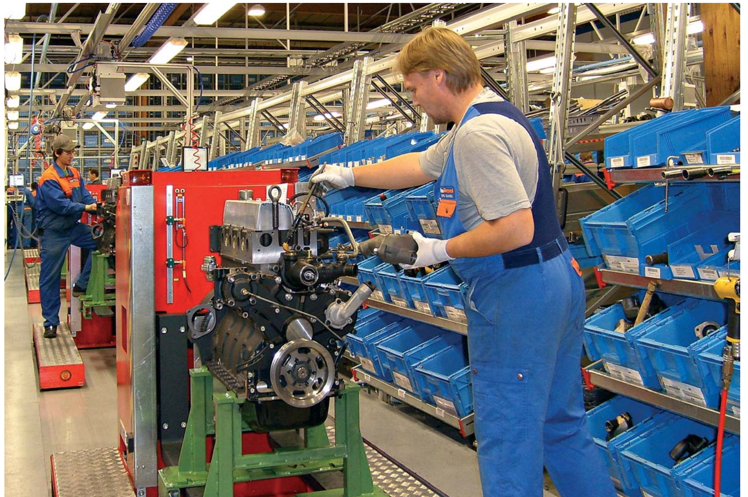
Ten AGVs are used in the final assembly of diesel engines at Sisu Diesel, Finland. Page 3.
