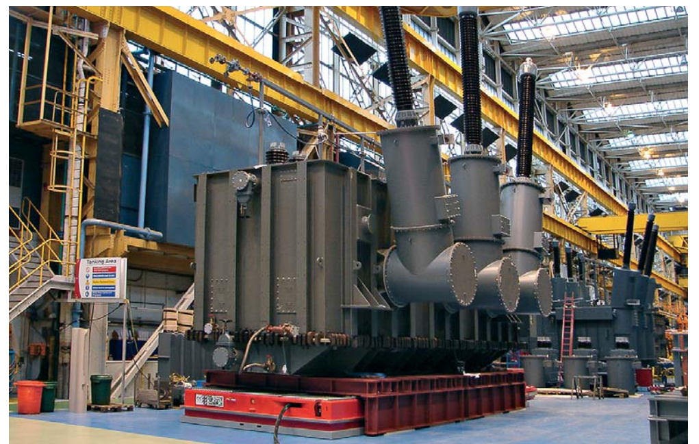
Fully-assembled transformers weighing up to 540 tonnes are moved into the test department using an Air Film Mover system.
